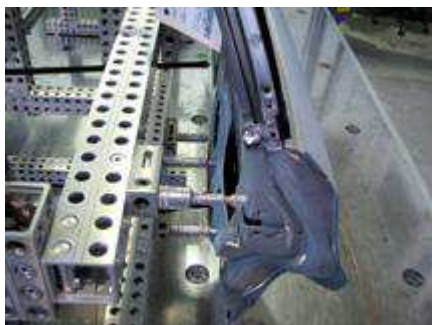
A close-up view showing a three-axis adjustable locating element holding a door in body position.
