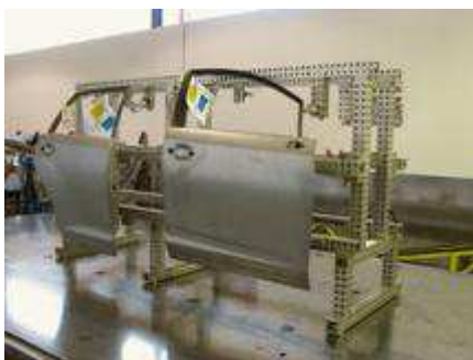
Two sided modular tool converted for reuse after its initial run for a different manufacturer.
